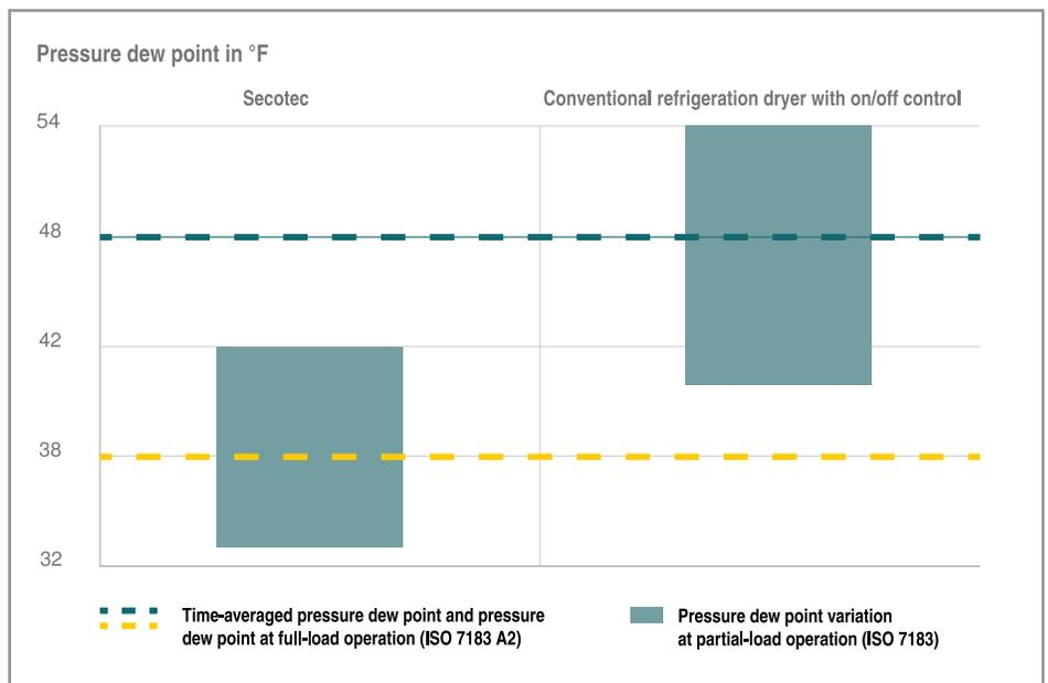
drying performance. This can be risky, since corrosion can take hold even with relative compressed air humidity of 40% – corrosion can therefore occur even without condensate formation. SECOTEC refrigerated dryers, on the other hand, ensure long-life operation thanks to their
